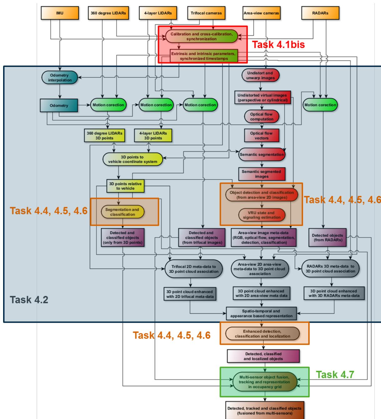
Figure 4 - Software architecture of the perception module (Task 4.1)
