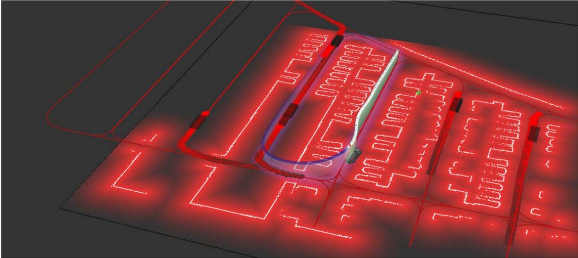
Figure 7 - Simulation environment. Ego vehicle is shown in blue, other vehicles are dark red and static obstacles are glowing red.
