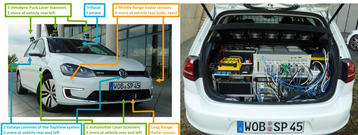
Figure 3 - Car with integrated sensors and the computer system
